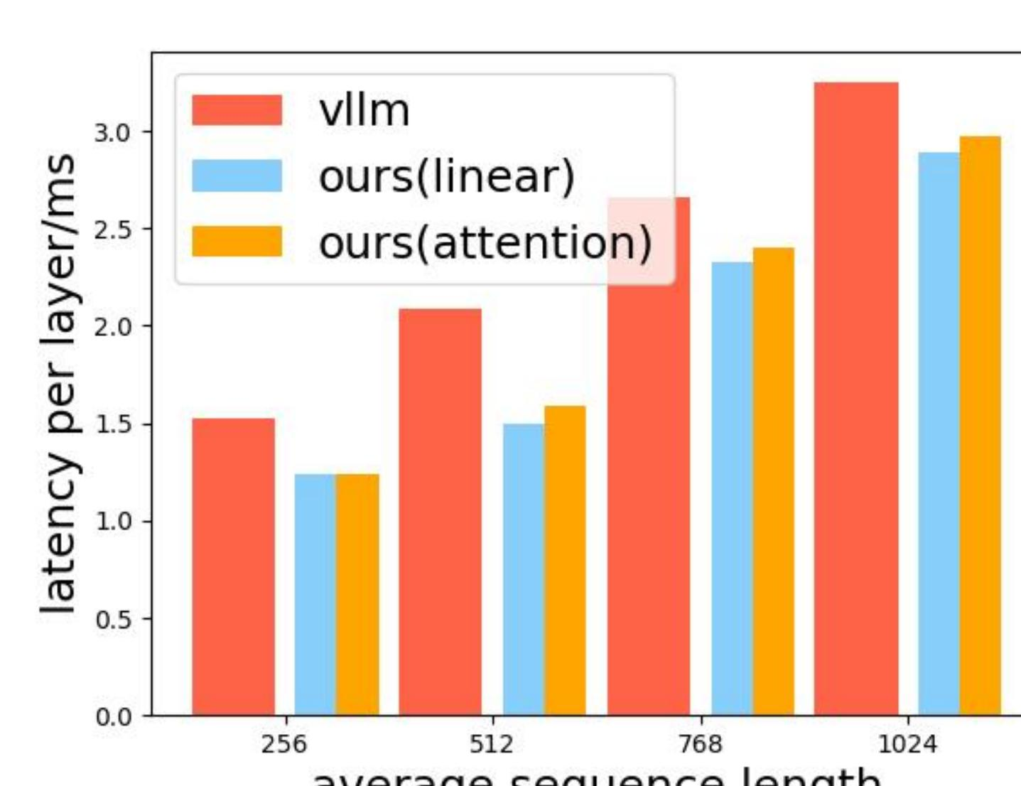
We prototyped PipeDecode on NVIDIA GTX 4090, and evaluated it with layers of Llama-7B model, a widely used open-source LLM.
